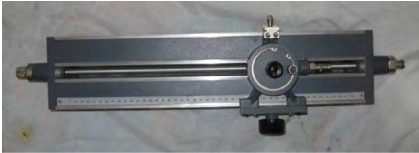
Figure 12.8: A slotted-line equipment which consists of a coaxial waveguide with a slot opening at the top to allow the measurement of the field strength and hence, the voltage standing wave pattern in the waveguide (courtesy of Microwave101.com).
